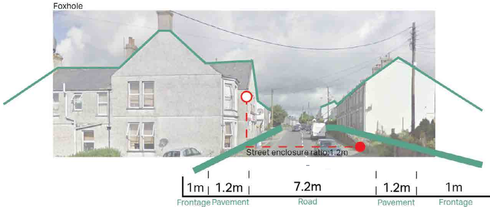
Figure 70: Diagram to demonstrate typical street dimensions and enclosure ratio.
