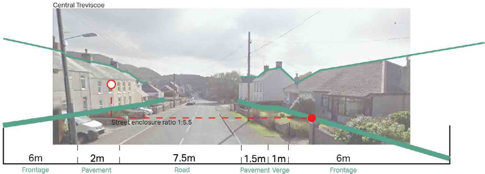
Figure 30: - Diagram to demonstrate typical street dimensions and enclosure ratio.
