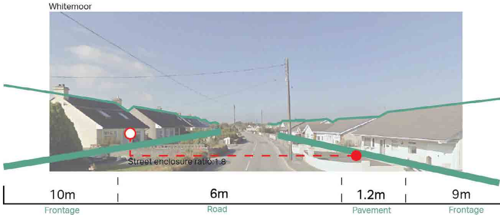
Figure 86: Diagram to demonstrate typical street dimensions and enclosure ratio.
