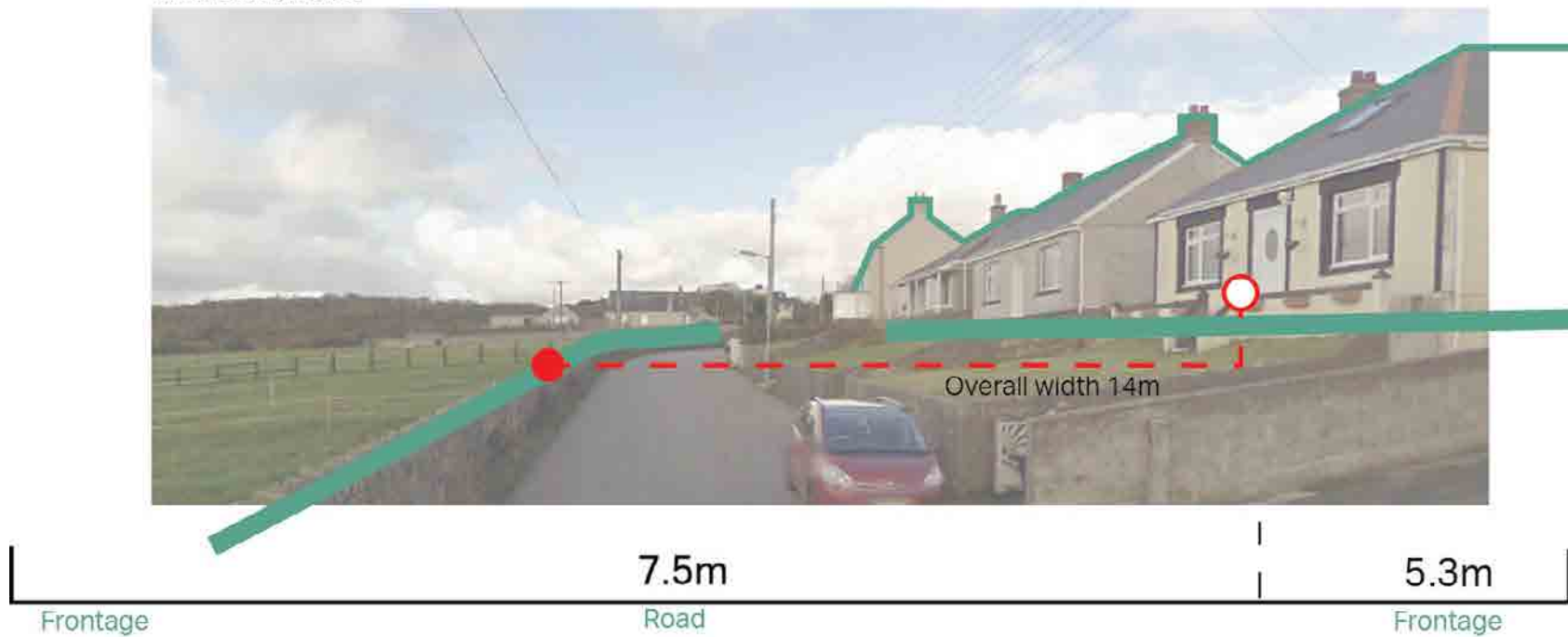
Figure 94: Diagram to demonstrate typical street dimensions and enclosure ratio.
